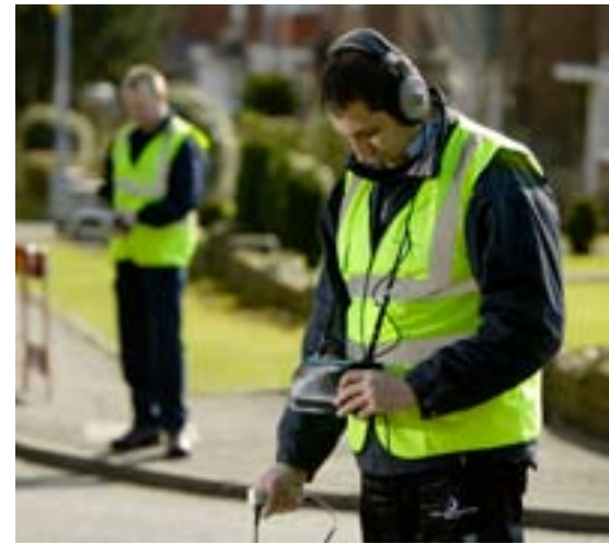
Leakage detection equipment
